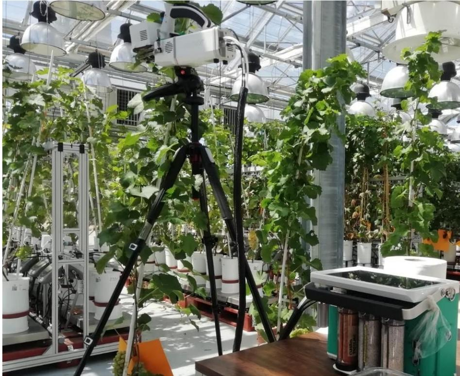
*Fig. 4: Licor 6800 which analyzes the photosynthetic and stomatal response.*
